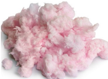
Loose fiberglass (itchy) - a good chance for mold growth
