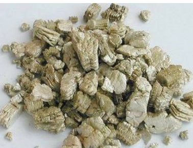
Vermiculite - contains asbestos HEALTH HAZARD not conducive to mold growth
